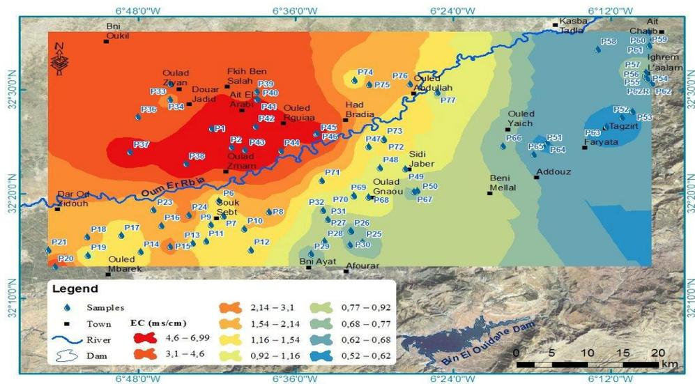
Figure 5: Variations of the Electrical Conductivity.
